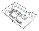
② Push the top of the USIM card to slide it out in the arrow direction,
