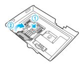
3 Lock the storage card holder by pushing it down into place.
