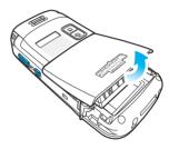
2 Lift off the battery to the arrow direction.
