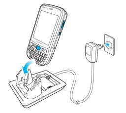
As you see in the picture, connect the adapter with the power cable to charge the PDA.
