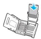
② Insert the microSD card into the storage card holder with its gold contacts facing out,
